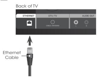
If you have a high-speed Internet connection, connect an Ethernet cable from your modem/router to the back of the TV as shown.
